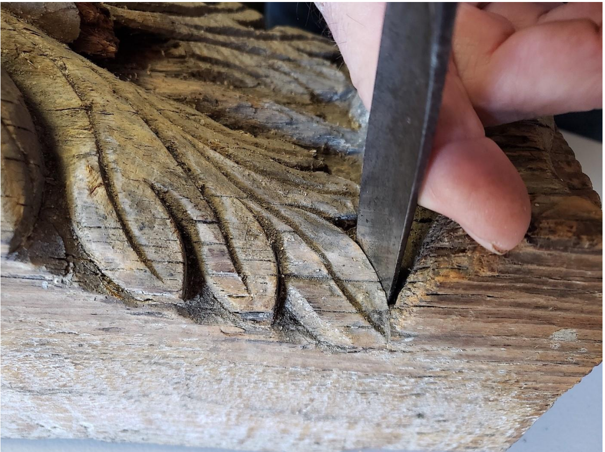
Figure 14. How gouge #5-20mm could be used to set-in a leaf of the finial.
