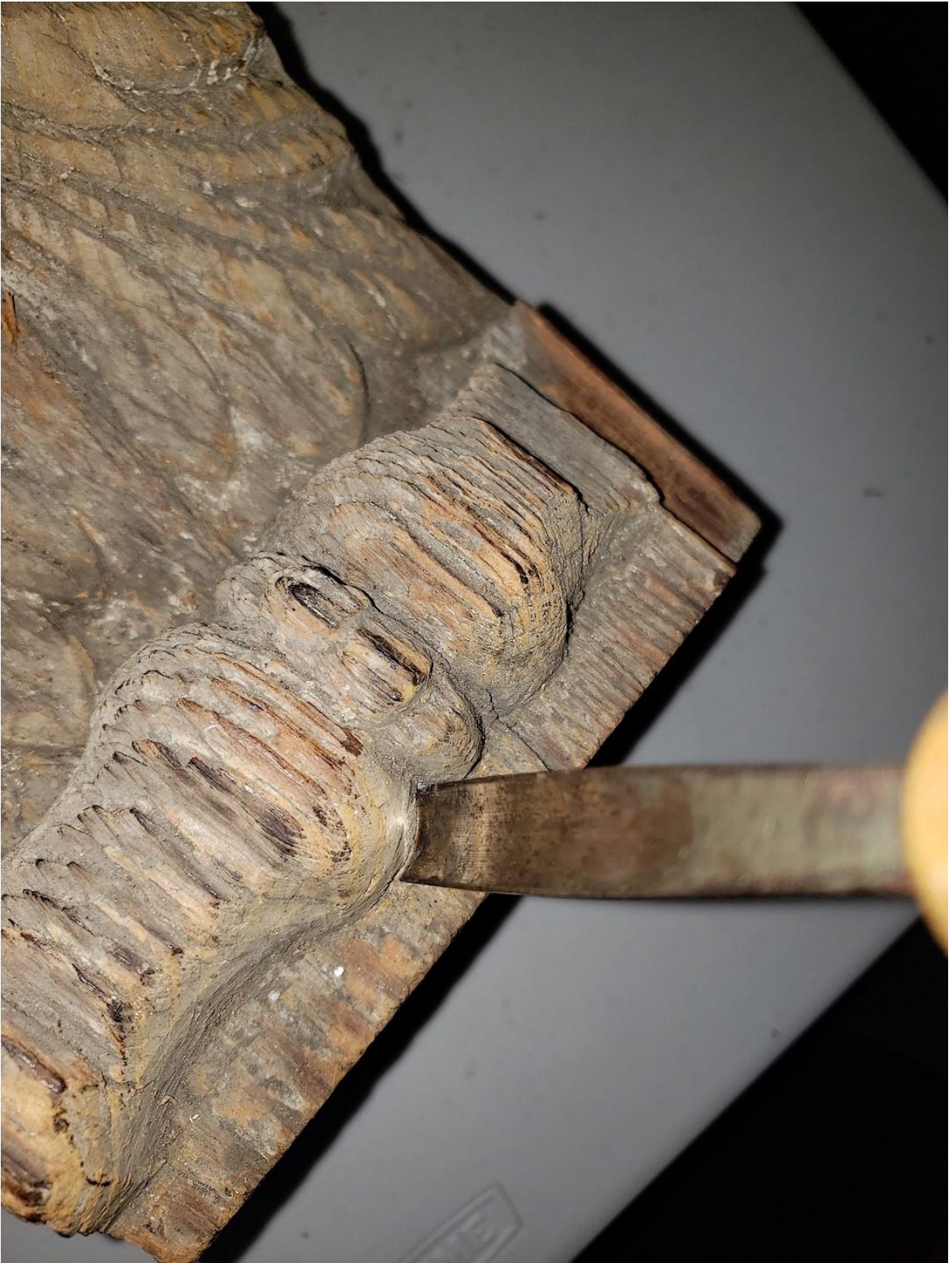
Figure 16. How gouge #7-14mm could be used to replicate the finial's lower vase-like elements.
