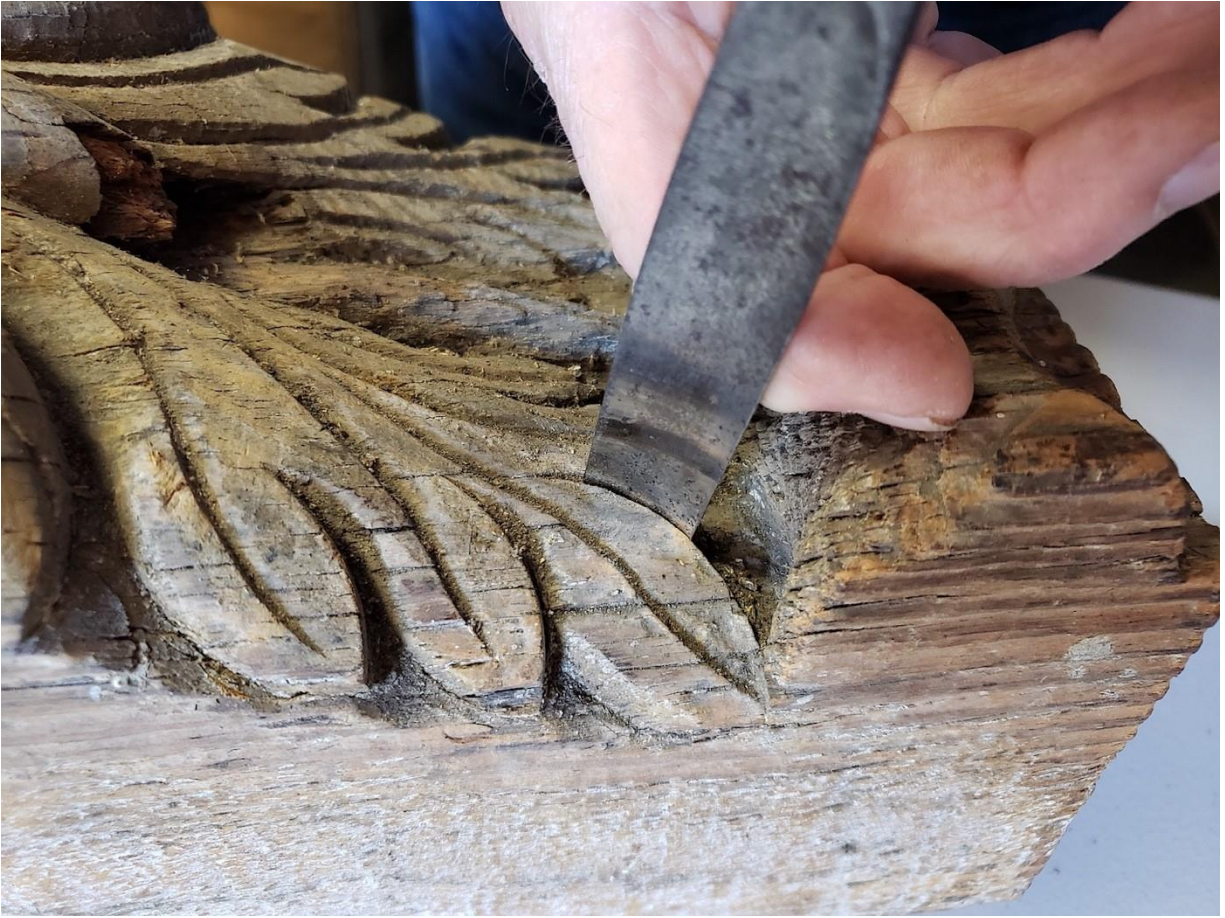
Figure 15. How gouge #5-20mm could be used to set-in a leaf of the finial.
