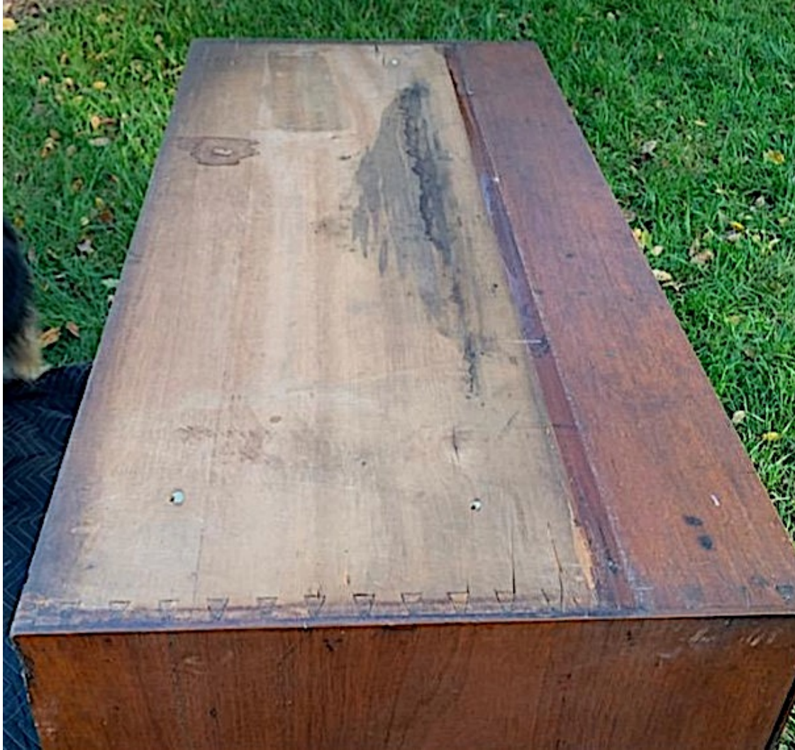
Figure 28 Top of chest portion of Fig. 22 (White dots are the screw holes for securing the bookcase.).
